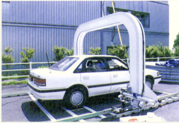
図13 自動車電話アンテナ周囲電界測定風景 Figure 13 Measurement of Spatial E-Field Distribution Emitted by Car-Phone Antenna.
