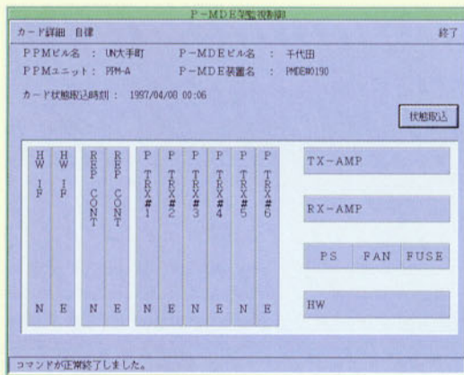
図5 P-MDE架監視画面 Figure 5 P-MDE Frame Monitoring Display.
