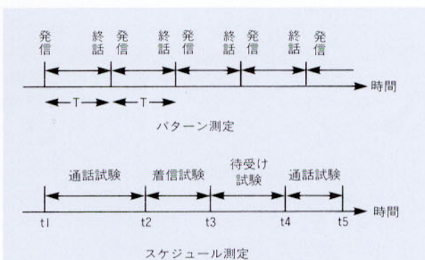
図7 パターン測定、スケジュール測定例 Figure 7 Example of Patterned and Scheduled Measurements
